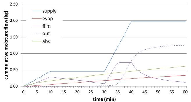
Fig. 8. Cumulative moisture flow on a concrete wall during a two shower rain event, including runoff, with catch ratios from Blocken and Carmeliet (2006).
