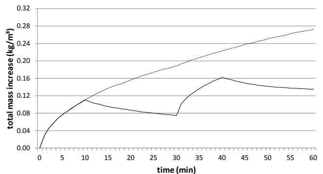
Fig. 9. Total mass increase of the wall during a two shower rain event with catch ratios from Blocken and Carmeliet (2006) with (dotted line) and without (full line) including runoff.
