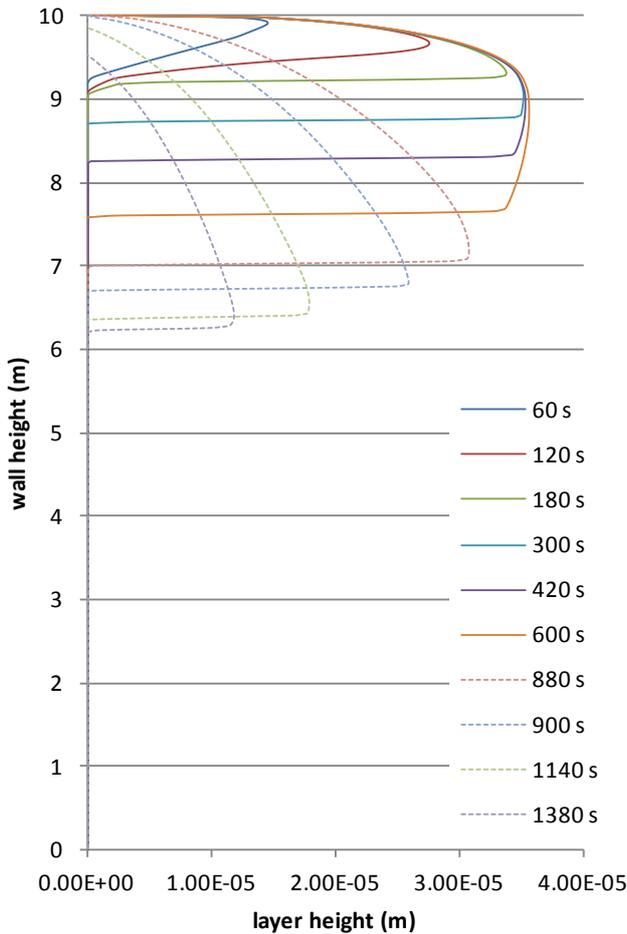
Fig. 5. Height of the runoff layer on a concrete wall during the first shower for a concentrated moisture load at the top of the wall. (full lines: growth of the layer, dotted lines: drying phase) at different stages.
