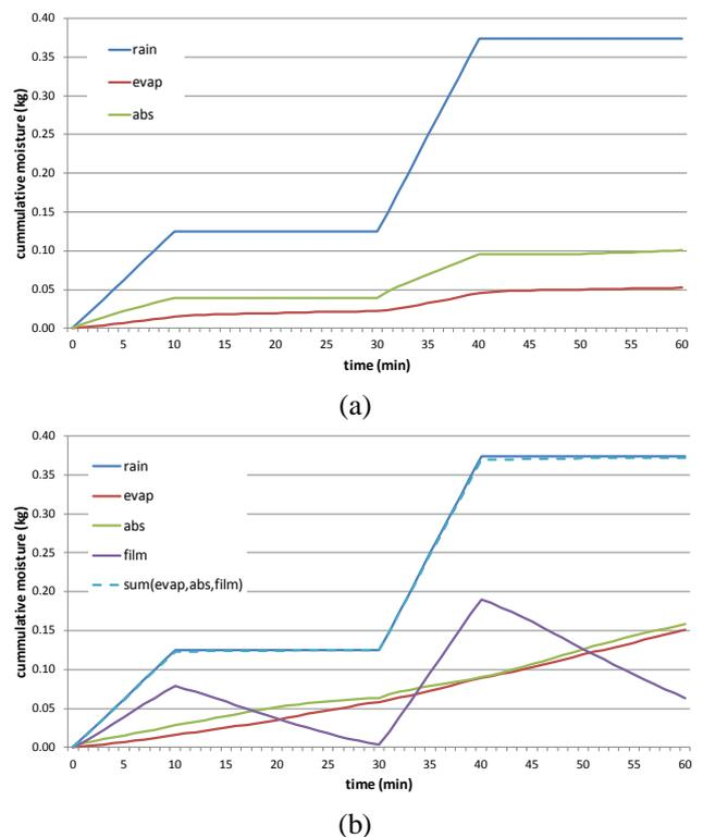
Fig. 4. Cumulative moisture flow on a concrete slab, without (a) and with (b) including runoff, during a 2 shower rain event for a concentrated moisture load at the top of the wall.
