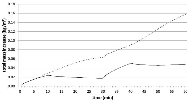
Fig. 6. Average moisture content of the concrete wall during a two shower rain event for a concentrated moisture load at the top of the concrete wall (dotted line: including runoff, full line: not including runoff).
