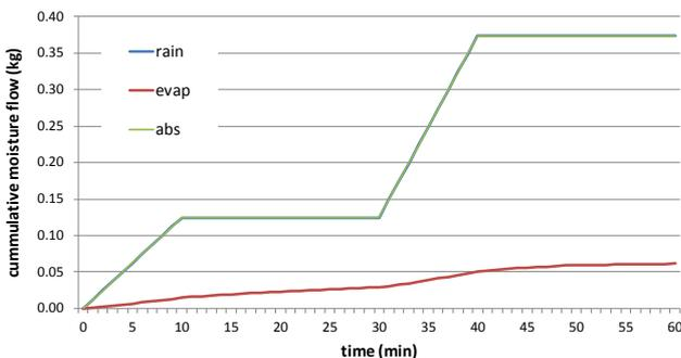
Fig. 7. Cumulative moisture flow on a brick wall during a two shower rain event for a concentrated moisture load at the top of the wall (case A).
