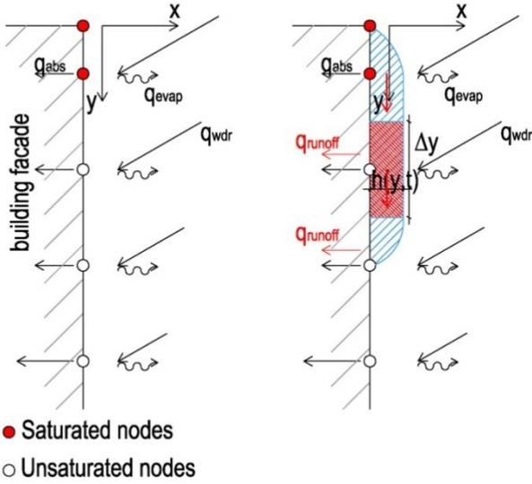
Fig. 2. Coordinate system and incoming flows of the coupled runoff model and HAM-model.
