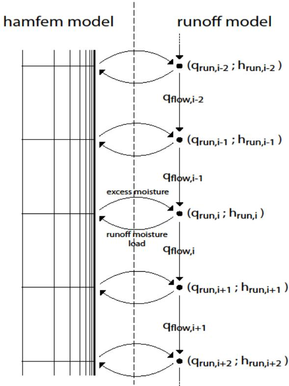
Fig. 1. Schematic representation of the coupled HAMFEM-runoff model. HAMFEM uses the amount of water in the runoff layer ( $q_{run,i}$ ) for input and returns the excess moisture that is used by the runoff model. The amount of vertical flow ( $q_{flow,i}$ ) and the height of the layer ( $h_{run,i}$ ) are used to evaluate the layer.
