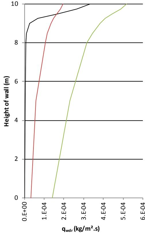
Fig. 3. Comparison of the wind driven rain from case A with case B, the catch ratios from Blocken en Carmeliet (2006) for a rain event with  $R_h = 1.2 \text{ mm/h}$  and  $U_{10} = 4.1 \text{ m/s}$  and a rain event with  $R_h = 2.4 \text{ mm/h}$  and  $U_{10} = 5.5 \text{ m/s}$ .
